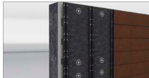
Mount the T-profile with approved fastening means
