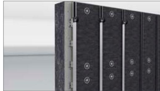
Apply joint tape on vertical bearing profiles
