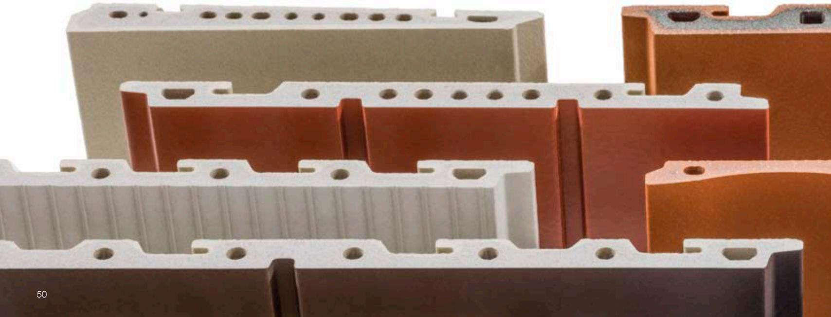
Extruded Ceramic Panels, Precision, DIN EN 14411, group Alla, glazed/unglazed (GL/UGL) (small-/large-size stoneware panels), 20 mm thick, 32 kg/m<sup>2</sup>
