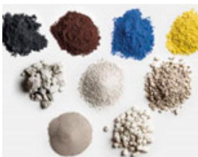
**Ceramics.** As a building material which has proved its value for thousands of years, ceramics displays ideal properties: it is non-combustible, resistant to chemicals, light-fast, resistant to pressure, impact and scratches, easy-care and hygienic.
