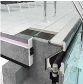
Large overflow channel with handhold-piece.
